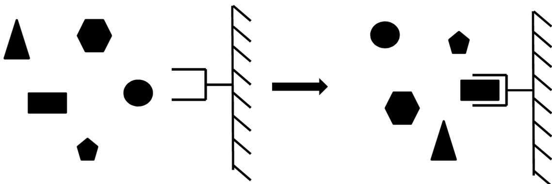
Figure 1: Lock-key principle for the removal of specific pharmaceuticals from the aqueous phase.
